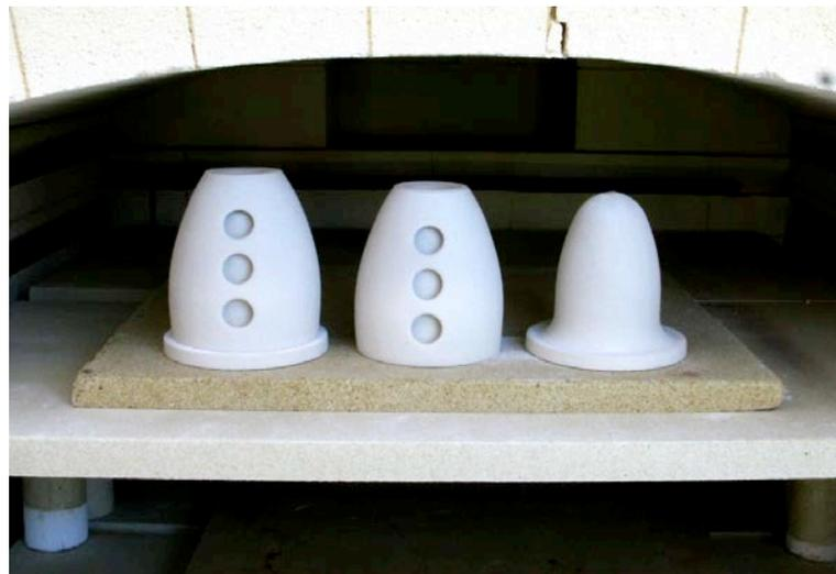
Figure 10 Beakers and setter in kiln
