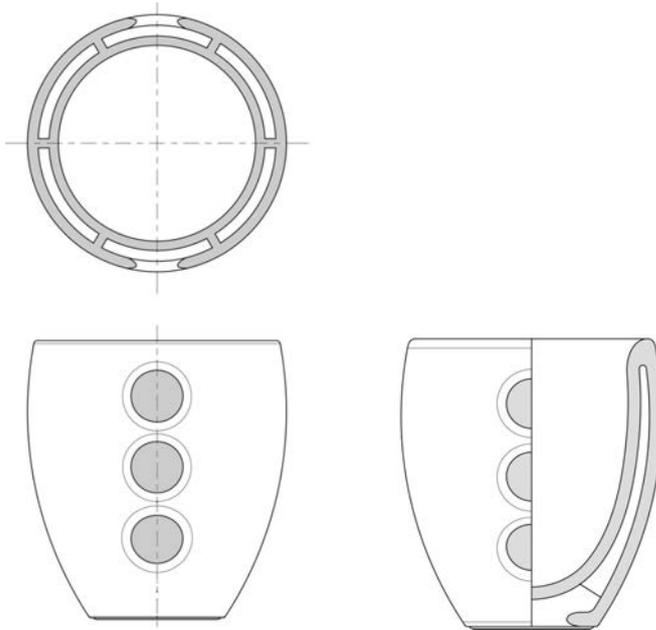
Figure 2 Double-walled ceramic beaker
