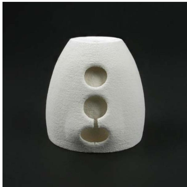
Figure 6 Firing the beaker on the setter significantly reduced distortion
