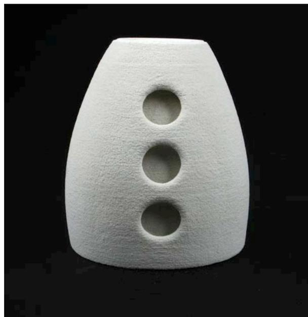
Figure 7 Distortion due to firing is further reduced due to increasing the size of the internal ribs of the beaker
