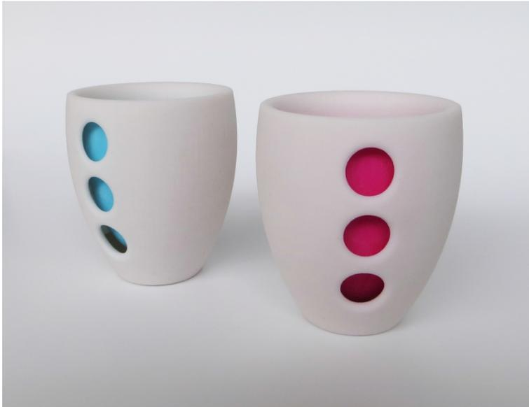
Figure 3 Beaker concept model in Z-Corp plaster-based modelling material.
