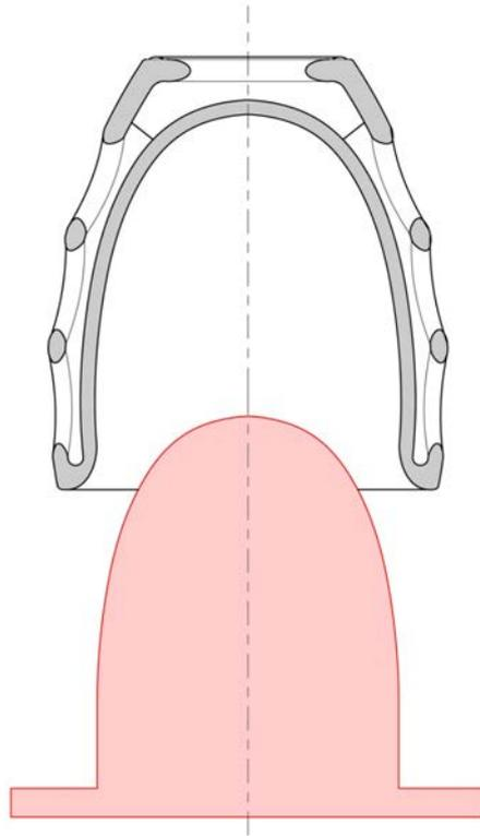
Figure 5 Design of the setter to support the beaker during firing
