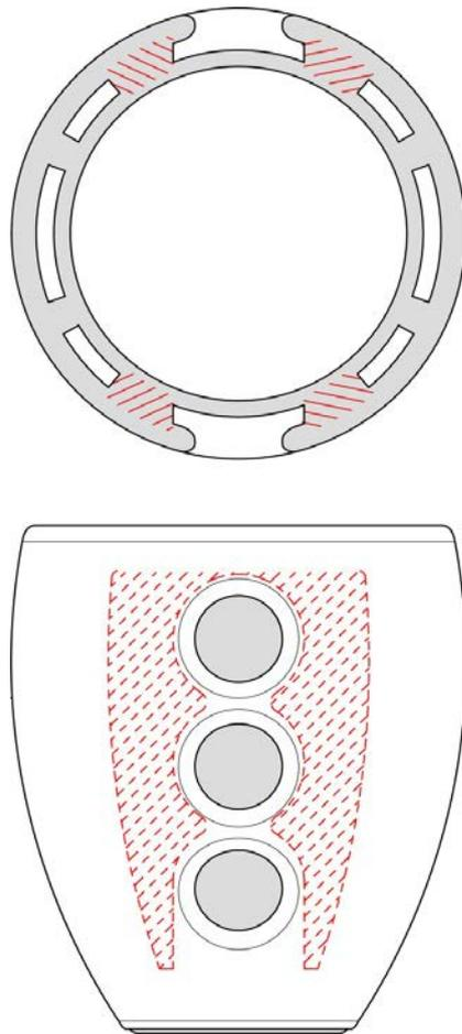
Figure 6 Increasing the size of the internal ribs of the beaker
