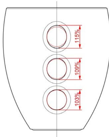
Figure 9 Stretching the beaker to compensate for vertical distortion.
