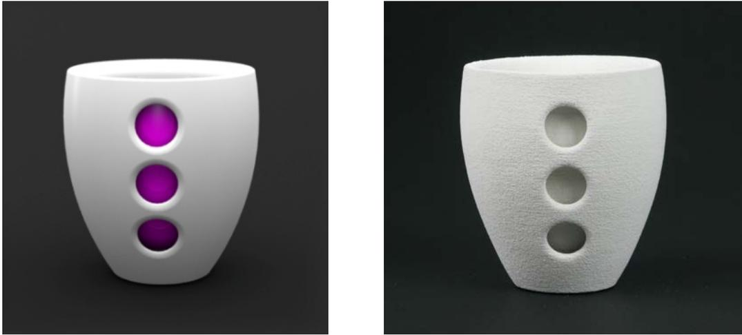
Figure 11 Biscuit fired ceramic beaker alongside 3D CAD model
