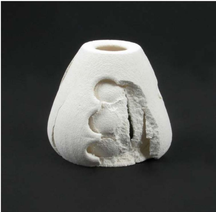
Figure 4 First attempt at firing the ceramic beaker without internal support
