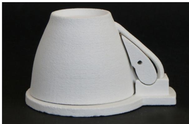
Figure 6 Cup and setter with handle support following firing
