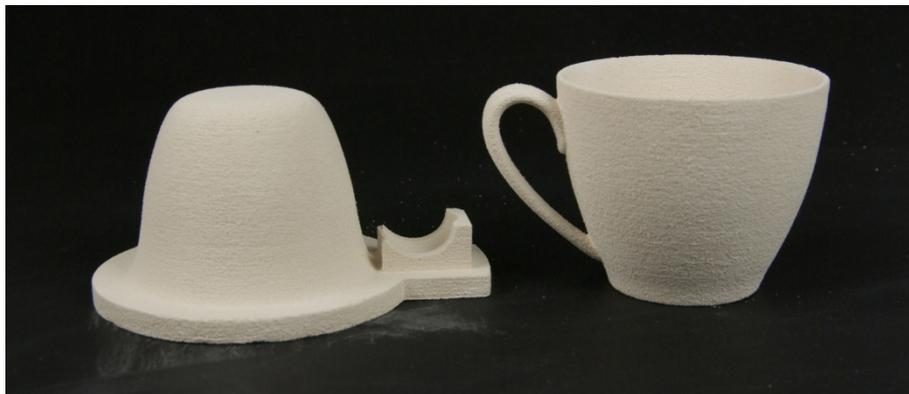
Figure 3 3D printed ceramic cup and setter prior to firing
