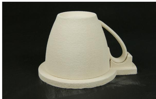
Figure 4 3D printed cup on setter prior to firing.
