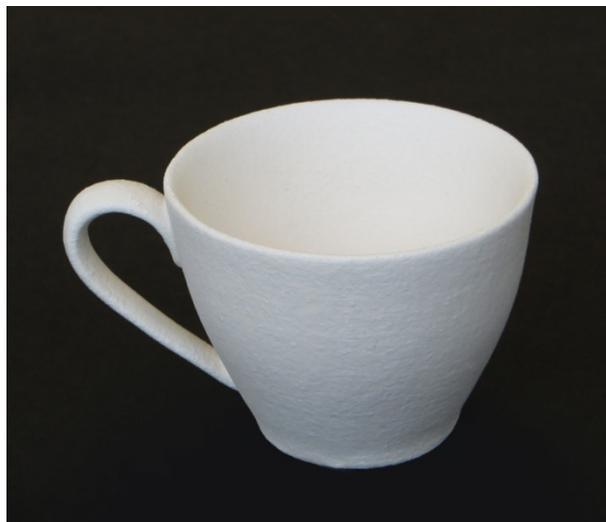
Figure 8 Finished cup with porcelain slip coating
