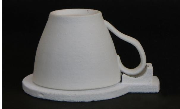
Figure 5 3D printed cup on setter following firing
