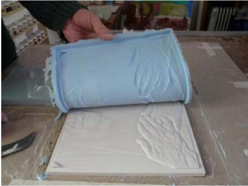
*Detail of rubber mould*
