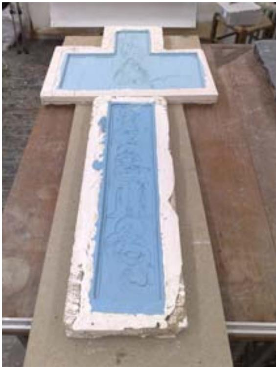
*Finished rubber mould*
