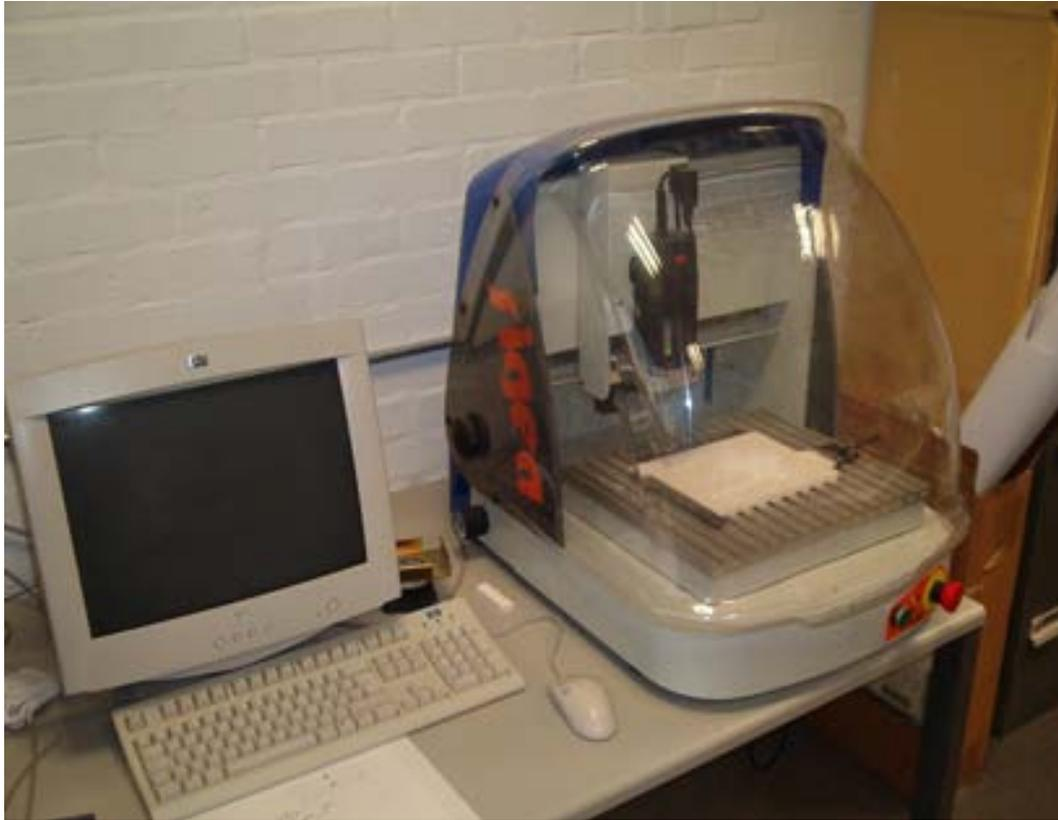
*Sigea Visio CNC machine milling plaster test block*
