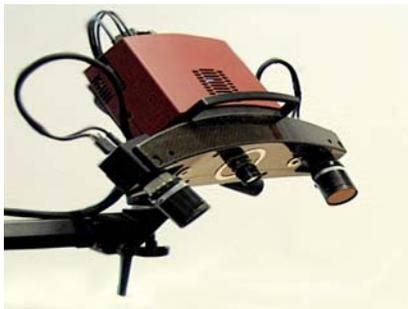
Fig, 2 Atos III white light scanner (courtesy of [www.gom.com](http://www.gom.com))
