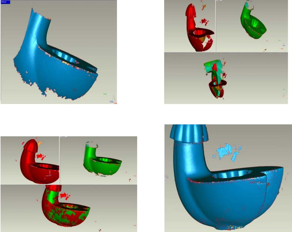
Fig. 8 merging scans in Geomagic
