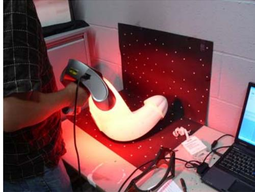
scanning the object using the handheld laser scanner
