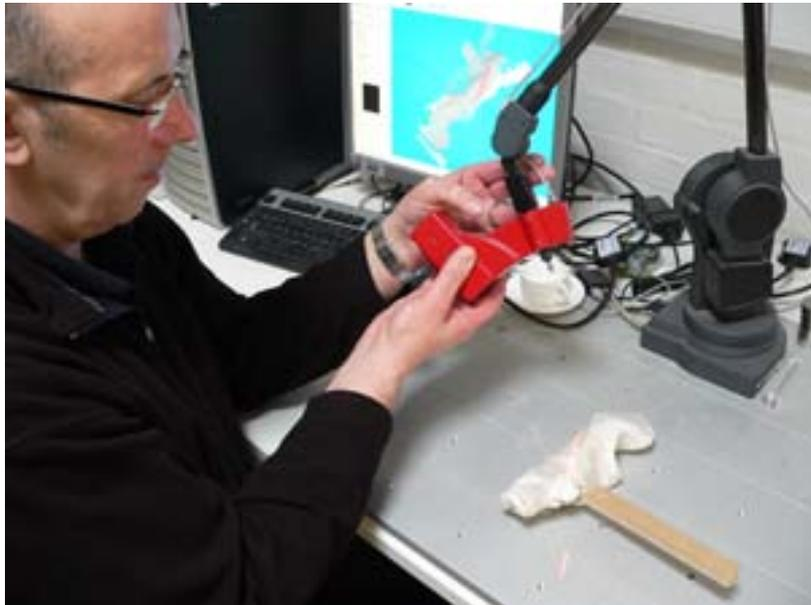
*3D laser scanning the clay impression*
