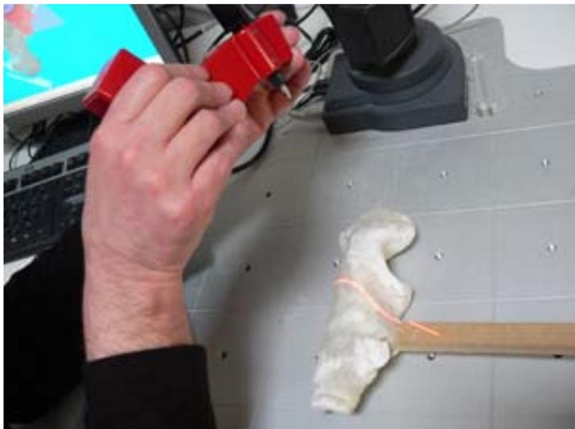
*3D laser scanning the clay impression*
