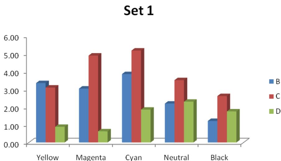
**Figure 10** dE between top surface, marked A, and respective other surfaces. Set 1 (Z-Corp 510, sanded, wax infiltration)
