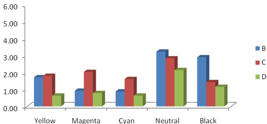
**Figure 13** dE between top surface, marked A, and respective other surfaces. Set 5 (Z-Corp 650, sanded, Z-Bond infiltration)
