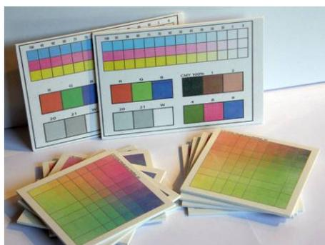
**Figure 2** 3D prints used for measurements, non-infiltrated sample presented (Stanic et al. 2008)
