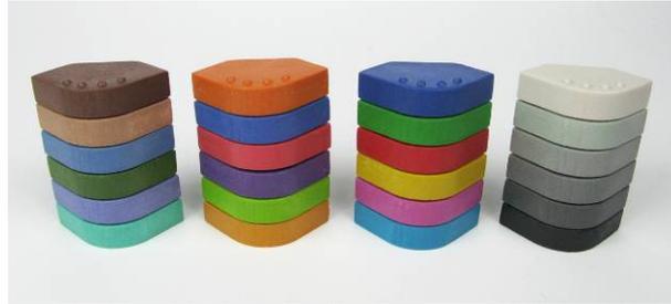
**Figure 7** 3D printed colour test blocks, which were built on the Z-Corporation Spectrum 510 3D printer, lightly sanded, and finished with Z-Bond infiltrant.
