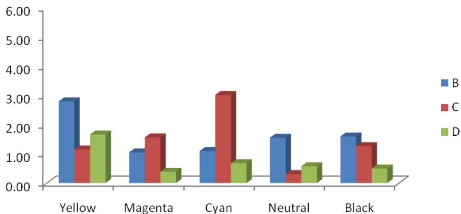
**Figure 12** dE between top surface, marked A, and respective other surfaces. Set 3 (Z-Corp 650, sanded, wax infiltration)
