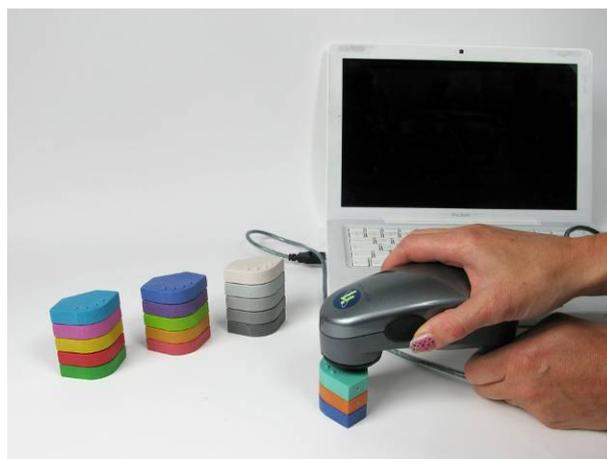
**Figure 9** Measurements were made using a GretagMacbeth EyeOne spectrophotometer
