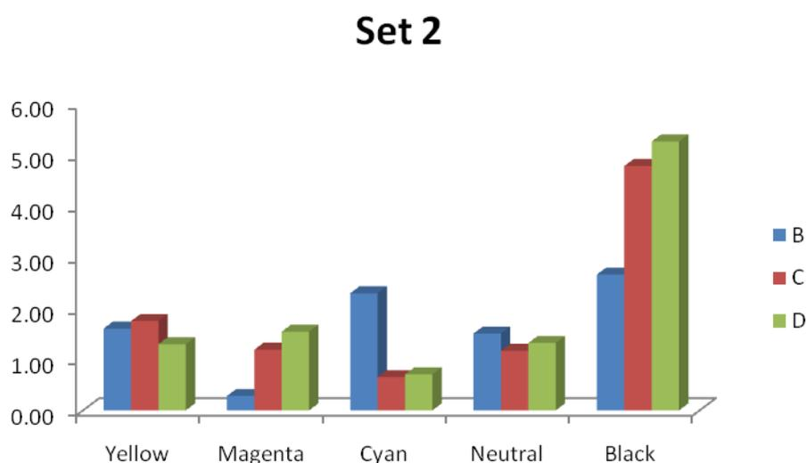
**Figure 11** dE between top surface, marked A, and respective other surfaces. Set 2 (Z-Corp 510, sanded, Z-Bond infiltration)
