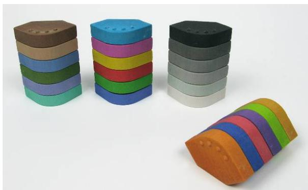
**Figure 6** 3D printed colour test blocks, which were built on the Z-Corporation Spectrum 510 3D printer, lightly sanded and then finished with wax infiltrant.
